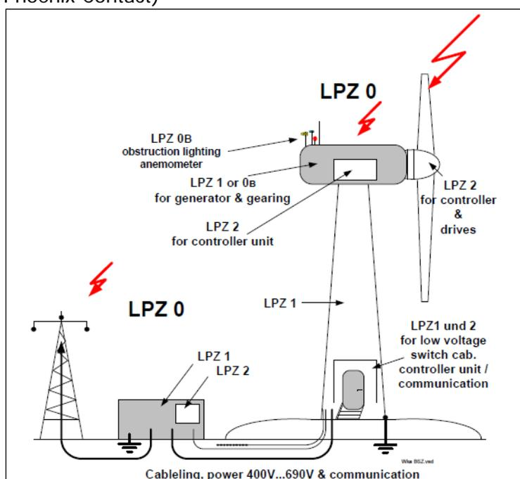
Attention has to be paid to the allocation of the wind turbines' components to individual lightning protection zones depending on the disturbance variable through partial lightning currents and switching surges that may be expected.
